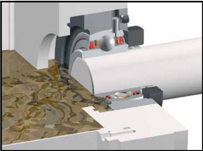
Simulation of Slurry Contamination Test
